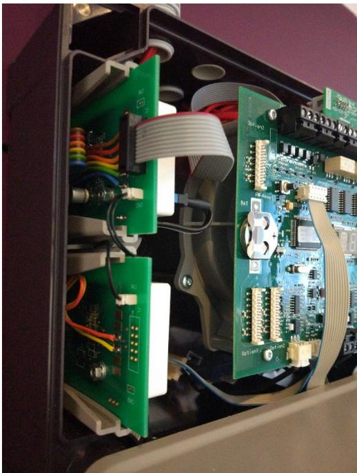
To install the SEC-HIM-35B, first install mounting bracket in the second slot and fasten with the Torx screw provided with the bracket.
