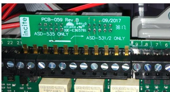
On the ASD535, install the board in terminals 10 to 20.
