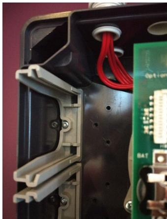
Locate and install the mounting bracket in the first slot and fasten with the Torx screw provided with the bracket.
