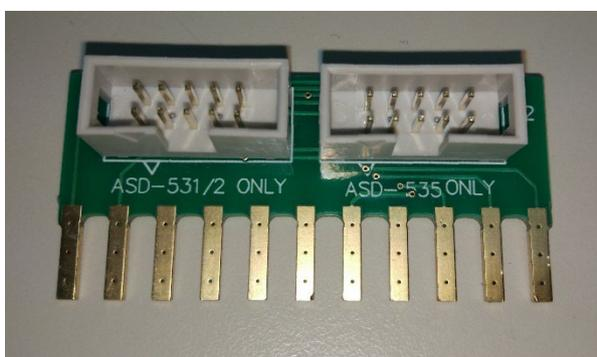
Locate the relevant plug for the type of ASD and connect the SEC-HIM-35.
