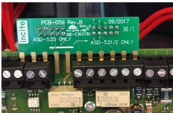
On the ASD531 and ASD532, install the board in terminals 8 to 16. Note the 2 fingers not connected.
